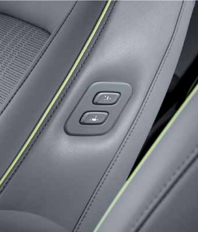
Passenger Seat Walk-in Device The passenger seat walk-in device means the driver or rear-seat passengers can adjust the front passenger seat to open up more cabin space.
