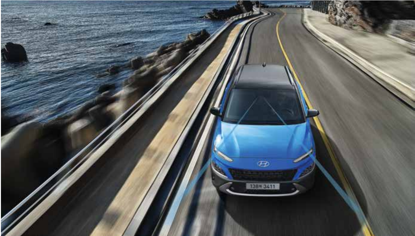
Lane Following Assist Helps with steering to keep the vehicle within the chosen driving lane.
