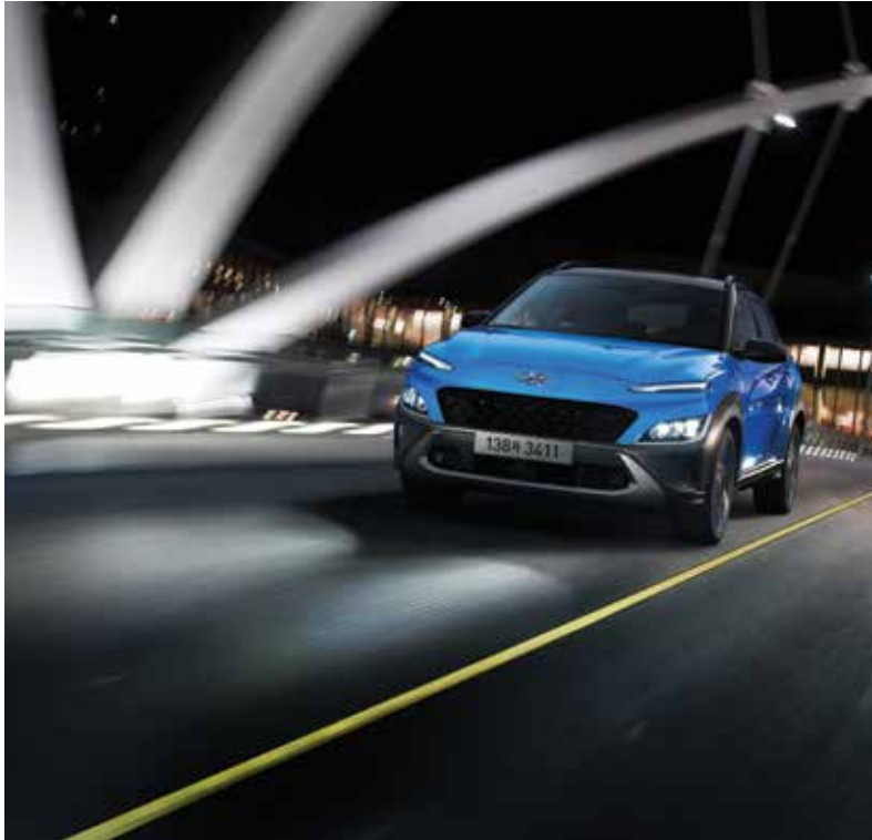
High Beam Assist Automatically switches high beams on or off in consideration of oncoming traffic while driving at night to reduce the need for adjustment, thereby protecting safety of the driver and of the people in oncoming vehicles.
