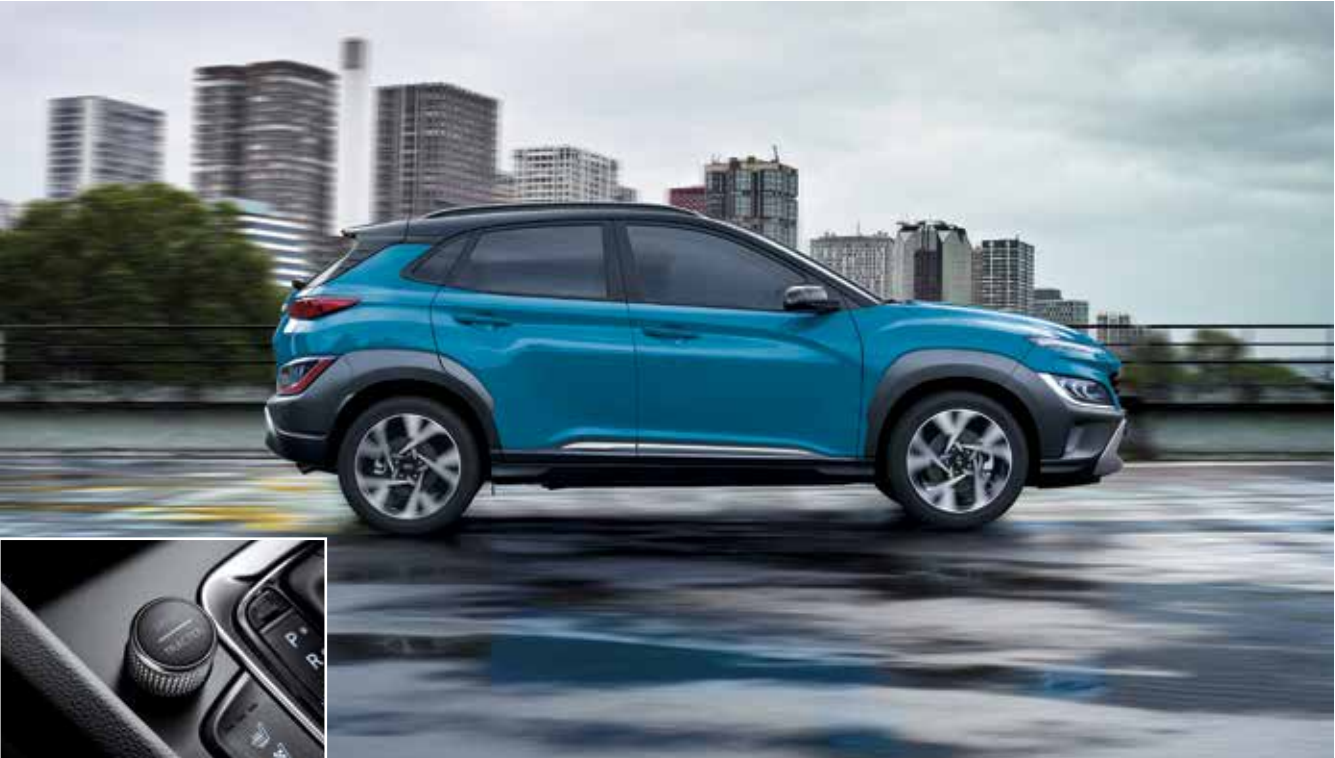
2WD Multi Terrain Mode Set your vehicle to multi-terrain mode with the traction mode's jog dial on the floor console. Turn the dial left or right to select driving conditions: Snow, Sand, or Mud. The engine and brakes then adjust to your selection for maximum performance on the surface conditions.
