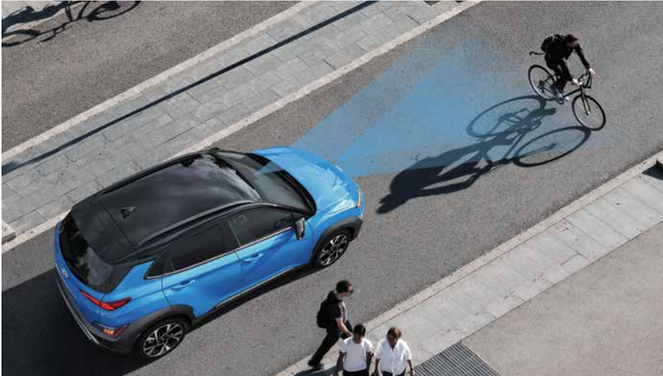
Forward Collision-Avoidance Assist Alerts the driver of the potential for a forward collision when vehicles in front suddenly slow down or stop, or pedestrians or cyclists appear in front of the vehicle. It also assists in activating brakes in the event of an impending collision.
