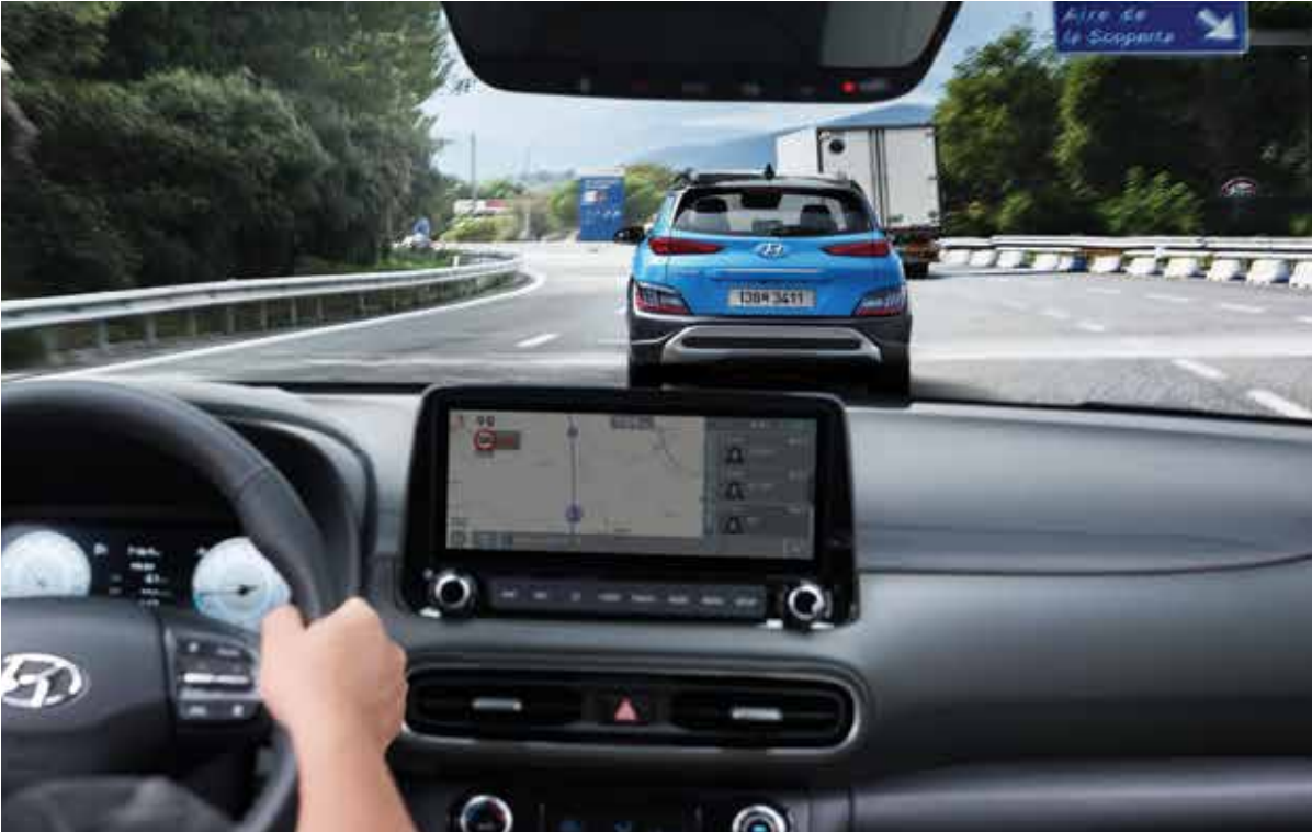
Navigation-Based Smart Cruise Control Ensures safe driving once it is switched on, by automatically adjusting vehicle speed on the highway. The smart cruise control recues vehicle speed automatically within safe driving zones and curved sections of the road and resumes back to the speed set by the driver once the vehicle exits such areas.
