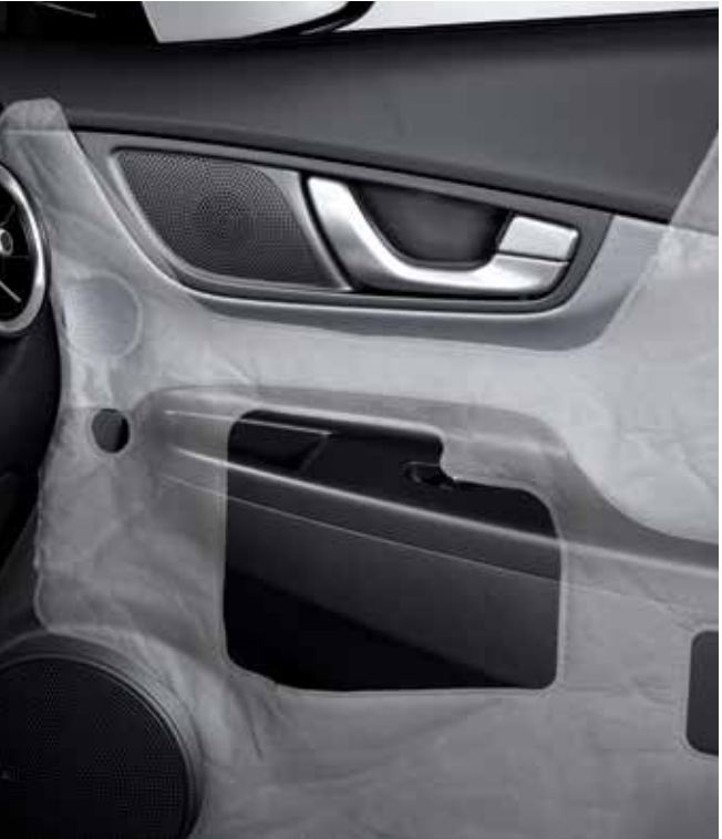
Reduced Road Noise Absorbent inside the doors, fillers, luggage trim, and wheel guards improve shielding of the interior and insulation from outside noise.
